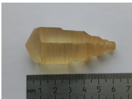
\text{LiRbMo}_3\text{O}_{10} single crystal grown in the [001] direction.
