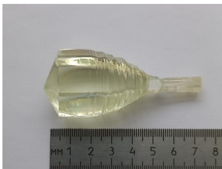
\text{NaCsMo}_3\text{O}_{10} single crystal grown in the [001] direction
