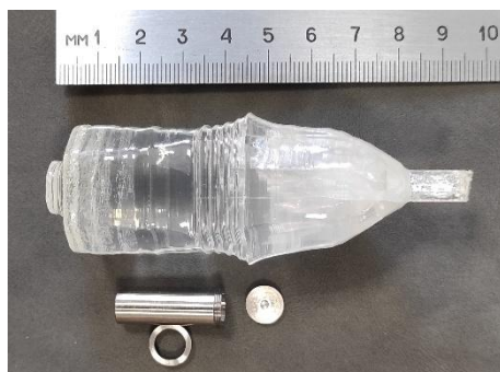
Gadolinium molybdate single crystal and titanium calorimeter container
