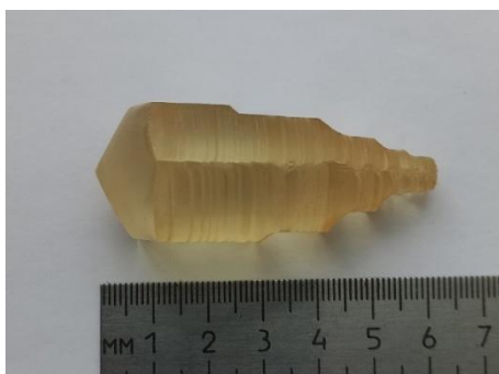
\text{LiRbMo}_3\text{O}_{10} single crystal grown in the [001] direction.
