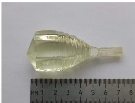
\text{NaCsMo}_3\text{O}_{10} single crystal grown in the [001] direction
